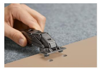
Thin door hinges are mounted using the EXPANDO T mounting method. Hinge cup drilling is no longer required, which makes the hinges suitable for very hard materials.
