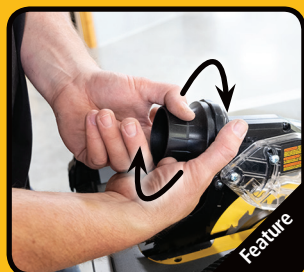
Twist adapter around port
