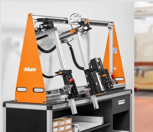
Using the new BOXFIX plus you can assemble TANDEMBOX and LEGRABOX faster than ever. Its easy setup, pneumatic clamps, and comfortable work height all contribute to faster, more efficient assembly of LEGRABOX and TANDEMBOX drawers.
