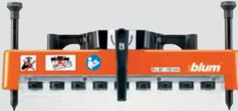
**NOTE:** Requires 5 each left hand and 4 each right hand drill bits. Recommended drill bit size for quick disconnect chucks: overall length is 57 mm and shank is 10 mm in diameter and 27 mm in length.
