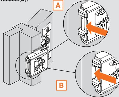
**Step 2:** While the CLIP lever is released, pull forward on hinge / door to remove from cabinet.
