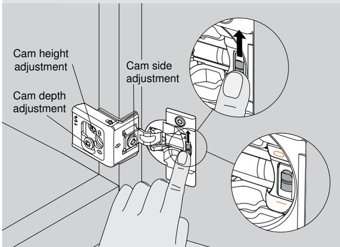
**NOTE:** COMPACT BLUMOTION comes in the activated position, marked with an "I" – the deactivated position is marked with a "0"
