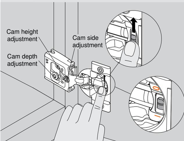
**NOTE:** COMPACT BLUMOTION comes in the activated position, marked with a "1" – the deactivated position is marked with a "0"
