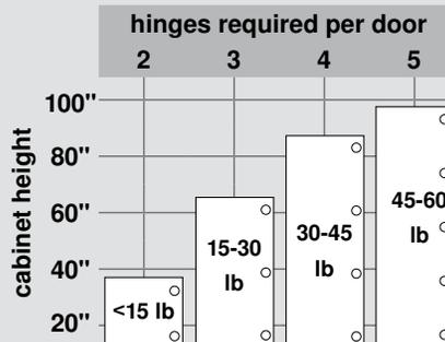
**NOTE:** The distance between the top and bottom hinges must be greater than the width of the door
