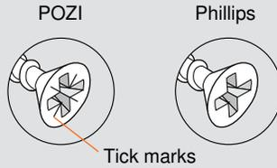
A POZI screwdriver (different from Phillips) is the most crucial tool you can use to assure that full torque is applied to all Blum adjustment screws. POZI screws can be identified by the distinctive "tick" marks located in the center of the screw head recess.
